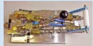
Depending upon the potlife of the material being sprayed and the hose lengths required, the mixing block can either be mounted on the frame of the proportioning unit or be externally located, directly where the spraying is taking place. Versions are available with either manual or automatically operated valves.
