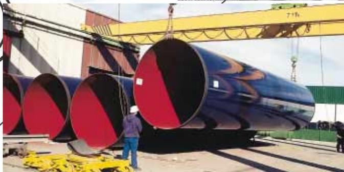
Here, pipes were sprayed with a polyurethane coating material (potlife: 30 seconds, spraying temperature: 55°C) using a WIWA DUOMIX 300.
