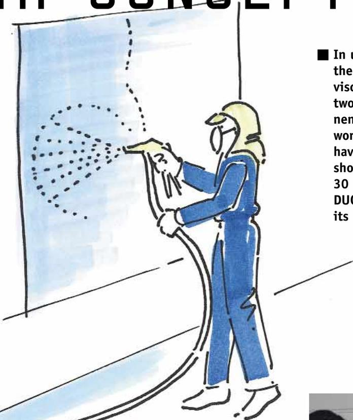
■ In use world-wide for the processing of high-viscosity, solvent-free two and three component materials. When working with materials having an extremely short potlife (i.e. 30 seconds), the WIWA DUOMIX best exhibits its strengths.
