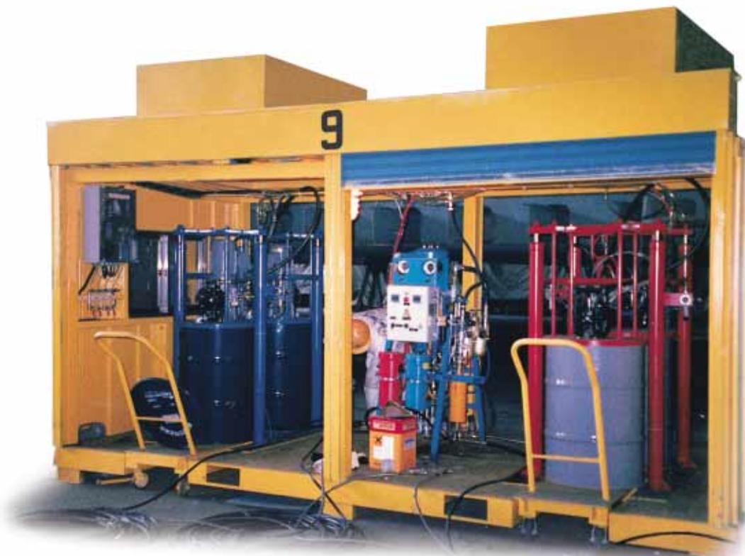
A complete WIWA DUOMIX Dual Component Unit, including an automatic drum refill system for both the base and hardener components, is integrated in a container, providing security, mobility and a maximum utilization of space. This enables the operator to quickly change locations within the wharf or on a shipdeck. Furthermore, the system is protected against climatic influences, as well as unauthorized access.
