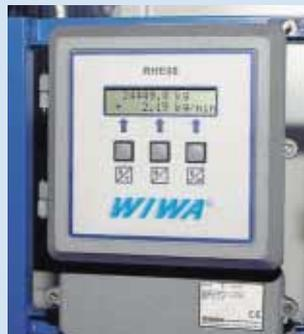
To measure the rate of flow of each component or to monitor the mixing ratio, various flow meters are available. The flow meters can be fitted with electronic analysis equipment, interfaces and printers to provide a written record of the measurement results.
