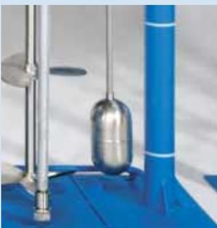
In order to achieve interruption-free operation of the WIWA DUOMIX Dual Component Spraying System, either a pneumatic or electric drum level indicator should be installed to monitor the amount of material remaining in each drum. When using the WIWA automatic drum refilling system, the feed drum is refilled automatically from a second drum once the level indicator registers that the minimum point has been reached.
