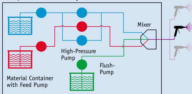
The high-pressure pump ensures that the exact dosage of each coating material component (base and hardener) is dispensed into the mixing block and then led to the spraying gun.
