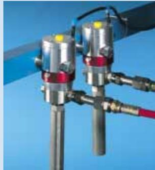
This assembly allows a small quantity of each component to be dispensed in an amount corresponding to the mixing ratio. These materials may then be mixed manually for touch-ups, which is very advantageous. No additional cleaning is necessary, as each component is dispensed separately.
