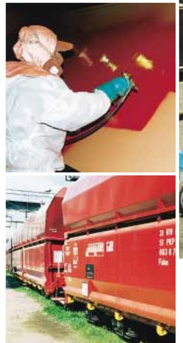
A railcar for transporting food is being coated with a solvent-free, thick polyurethane coating using a WIWA DUOMIX 333 (solids: 92,5%, potlife: 5 minutes, spraying temperature: 60°C).
